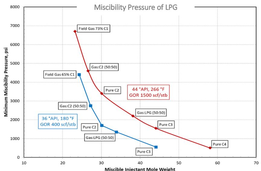
The pressure increase associated with the Single Shot IOR™ treatment, coupled with the energy associated with the post-treatment expansion of the LPGs as reservoir pressure drops, provides energy to drive incremental oil to the wellbore.
