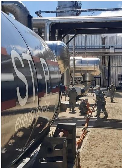
STEP recognized the potential for “shadow” zones within the process where LELs likely would have persisted due to a lack of turbulence. Understanding that these zones were going to be problematic allowed STEP to work with the client in the development of effective procedures to pressure cycle these areas and induce turbulence for improved vaporization of any remaining hydrocarbons.
